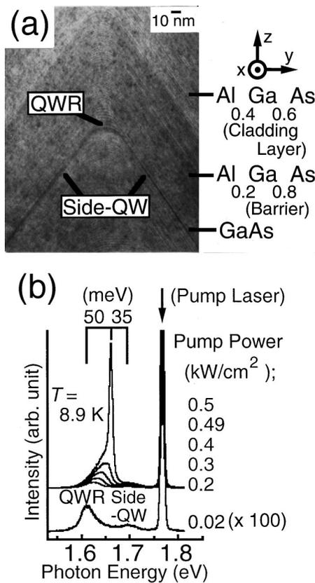
FIG. 1. (a) TEM cross-sectional image of a ridge QWR laser structure. The  $x$ ,  $y$ , and  $z$  directions are defined as the wire direction ( $x$ ), the lateral confinement direction ( $y$ ), and the growth direction ( $z$ ). (b) PL spectra at 8.9 K for the various excitation powers of 0.02, 0.2, 0.3, 0.4, 0.49, and 0.5  $\text{kW}/\text{cm}^2$ . The sharp line due to the stimulated emission was observed at 1.662 eV for 0.5  $\text{kW}/\text{cm}^2$ .
