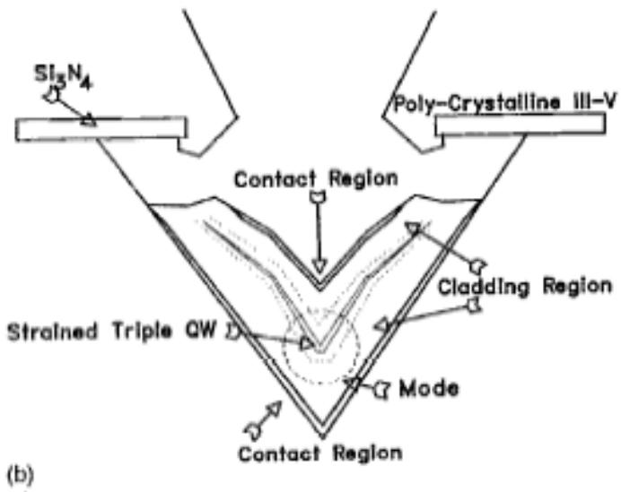
3-period V-groove QWRs with Si<sub>3</sub>N<sub>4</sub> mask
